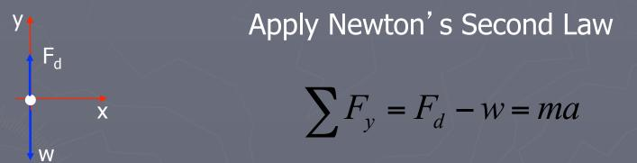
Where  $F_d$  is the magnitude of the drag force on the stone. This force is directed opposite the object's velocity.
